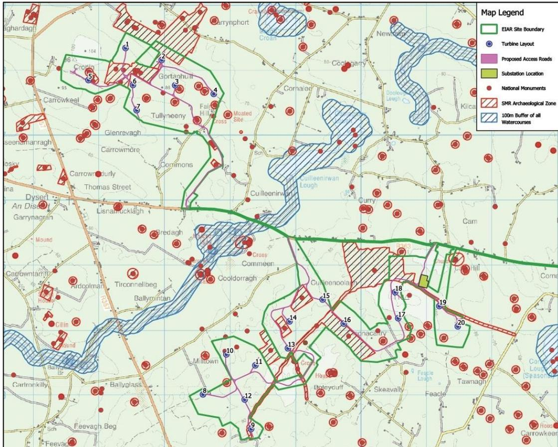
Figure 3-7 Fifth Site Layout (Revised 20 Turbine Layout Accounting for Archaeological, Geological and Hydrological Constraints)
