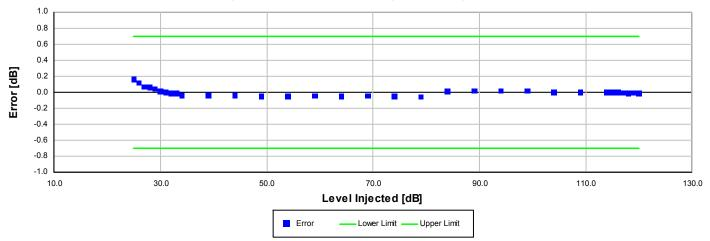
Broadband level linearity performed according to IEC 61672-3:2013 16 and ANSI S1.4-2014 Part 3: 16 for compliance to IEC 61672-1:2013 5.6, IEC 60804:2000 6.2, IEC 61252:2002 8, ANSI S1.4 (R2006) 6.9, ANSI S1.4-2014 Part 1: 5.6, ANSI S1.43 (R2007) 6.2
