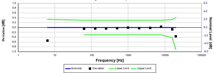
Electrical signal test of frequency weighting performed according to IEC 61672-3:2013 13 and ANSI S1.4-2014 Part 3: 13 for compliance to IEC 61672-1:2013 5.5; IEC 60651:2001 6.1 and 9.2.2; IEC 60804:2000 5; ANSI S1.4:1983 (R2006) 5.1 and 8.2.1; ANSI S1.4-2014 Part 1: 5.5
