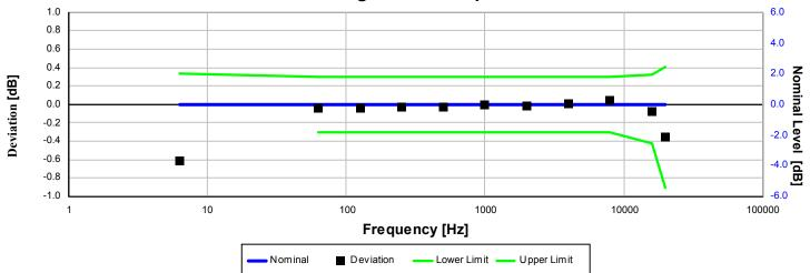
Electrical signal test of frequency weighting performed according to IEC 61672-3:2013 13 and ANSI S1.4-2014 Part 3: 13 for compliance to IEC 61672-1:2013 5.5; IEC 60651:2001 6.1 and 9.2.2; IEC 60804:2000 5; ANSI S1.4:1983 (R2006) 5.1 and 8.2.1; ANSI S1.4-2014 Part 1: 5.5
